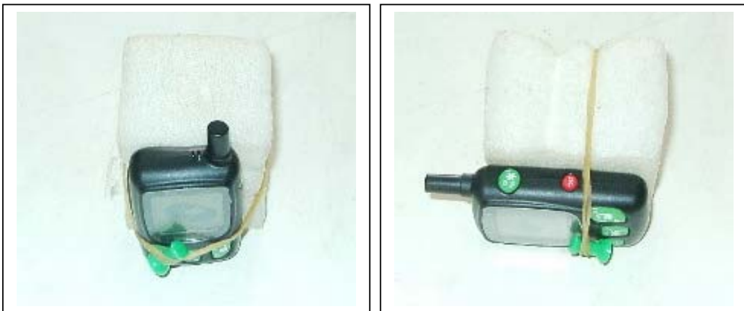
Radiated Open Site Test Set-up (Transmitter Mode)
