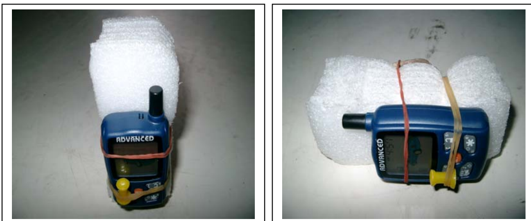
Radiated Open Site Test Set-up (Transmitter Mode)
