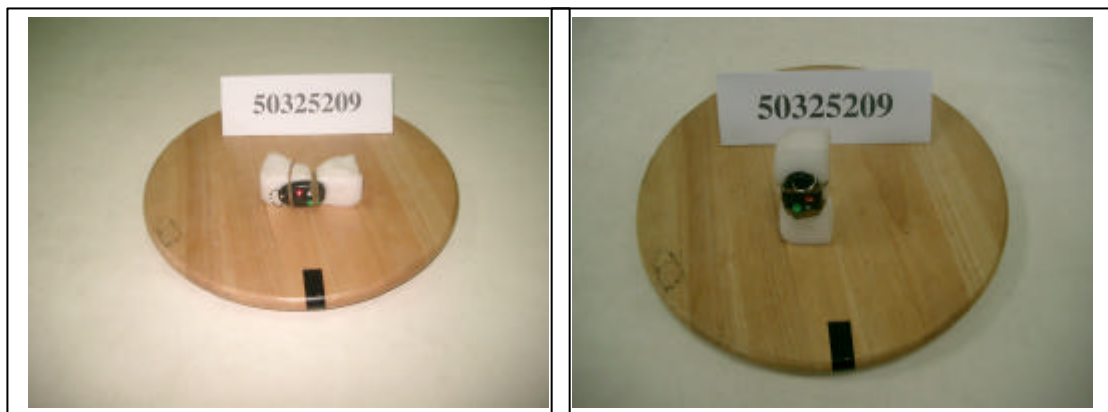
Radiated Open Site Test Set-up
