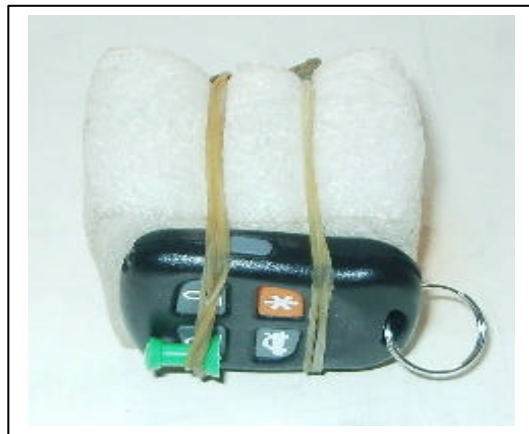
Radiated Open Site Test Set-up
