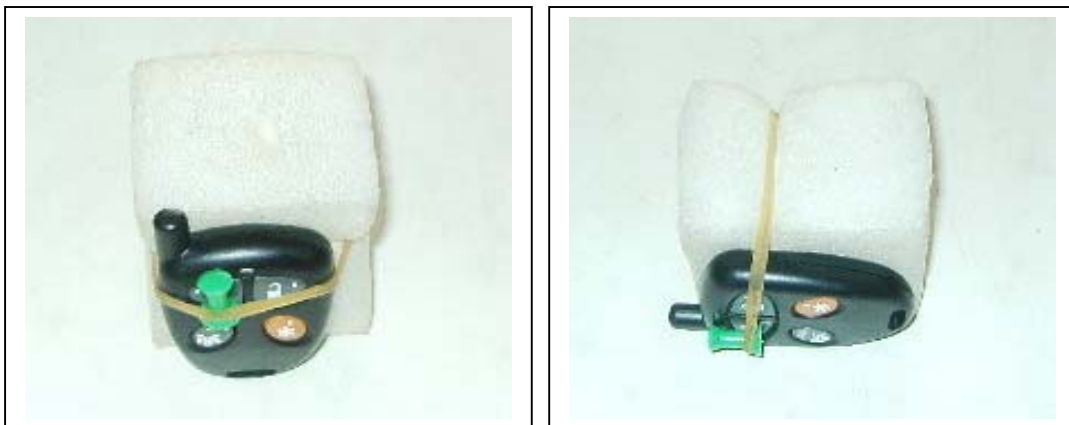
Radiated Open Site Test Set-up
