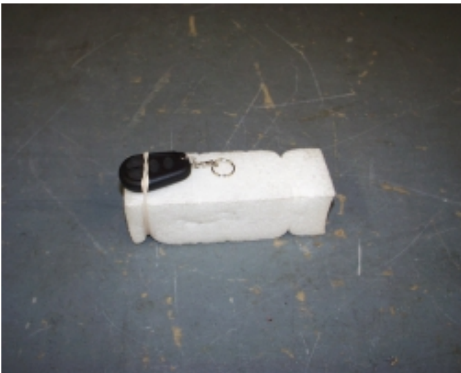
Radiated Open Site Test Set-up
