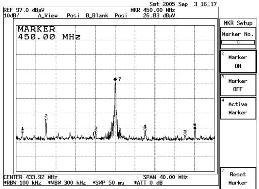
Number seven: Another transmitter trigger signal (62.48dB)
