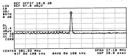
08:35:54 JUN 19, 1998 FCC ID: H5DR23 APP NEAR FIELD PROBE: RX 6AIN; ADVANCE SECURITY(302MHz RX ACTV DET: PEAK MEAS DET: PEAK QP AV6 MKR 302.01 MHz 77.64 dBµV
