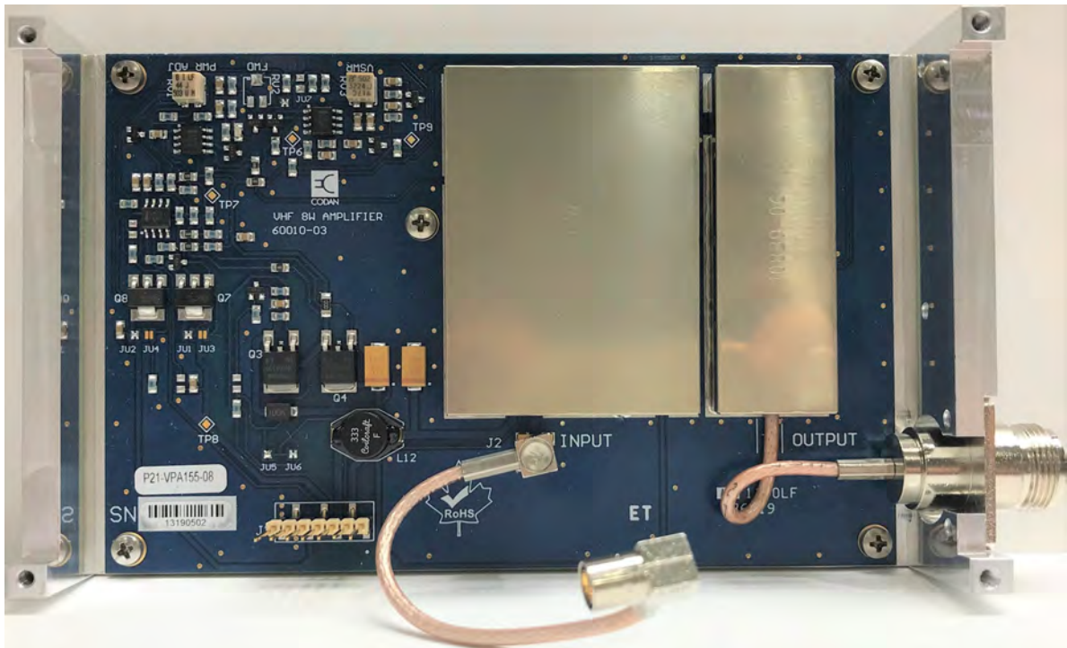
Power Amplifier Board – Top Side, Shields Installed
