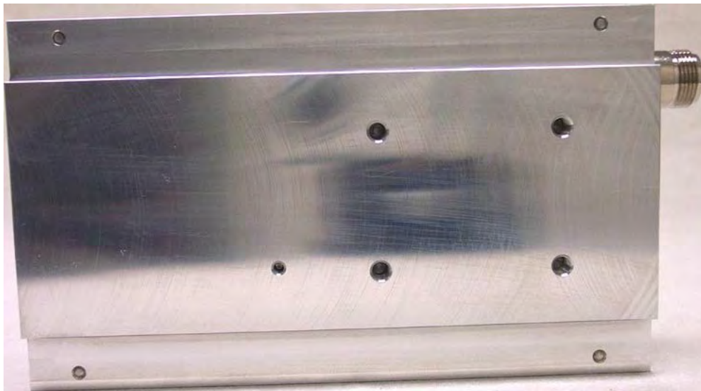
Power Amplifier – Heat-Sink Outside
