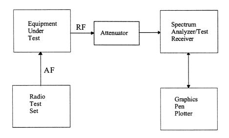
\* The transmitter was modulated with a 2500 Hz tone at an input level 16 dB greater than that necessary to produce 50% modulation. Spectrum Analyzer settings as per measurement data plot.
