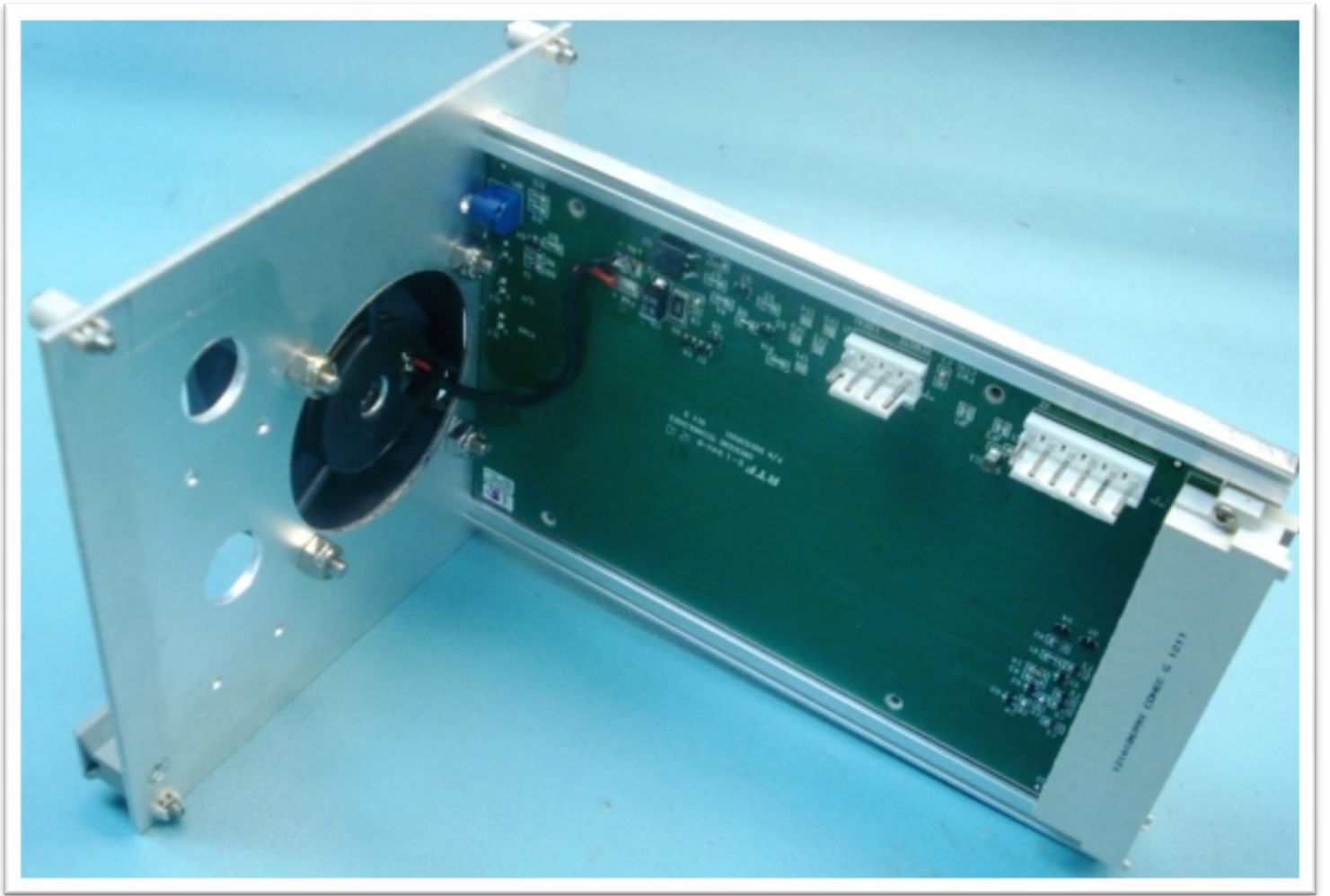
5 – Alarm Board & Front Panel
