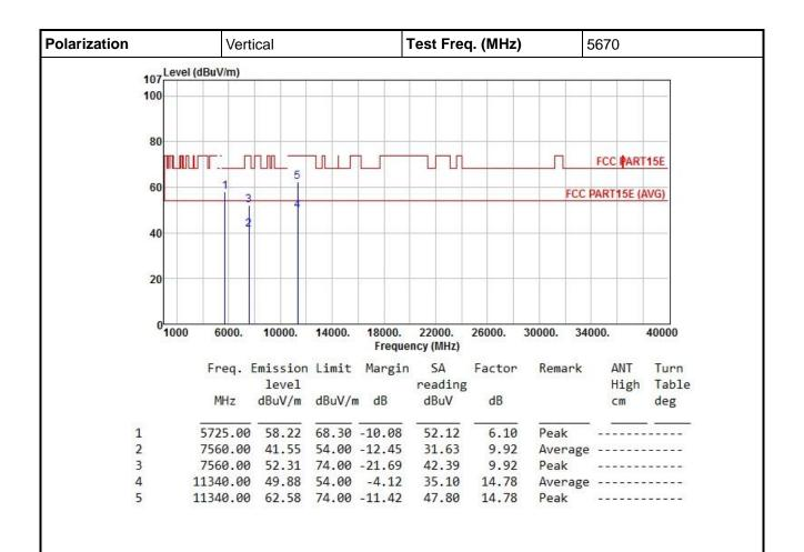
Note 1: ">20dB" means spurious emission levels that exceed the level of 20 dB below the applicable limit. Note 2: For restricted bands, the peak measurement is fully sufficient, as the max field strength as measured
