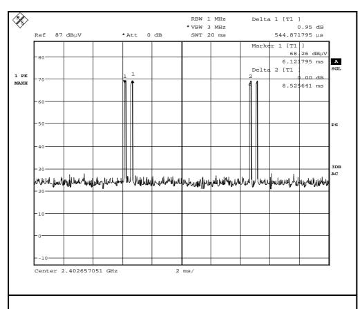
$20 \log (Duty cycle) = 20 \log (0.2 \text{ ms} / 8.526 \text{ ms}) = -32.6 \text{ dB}$
