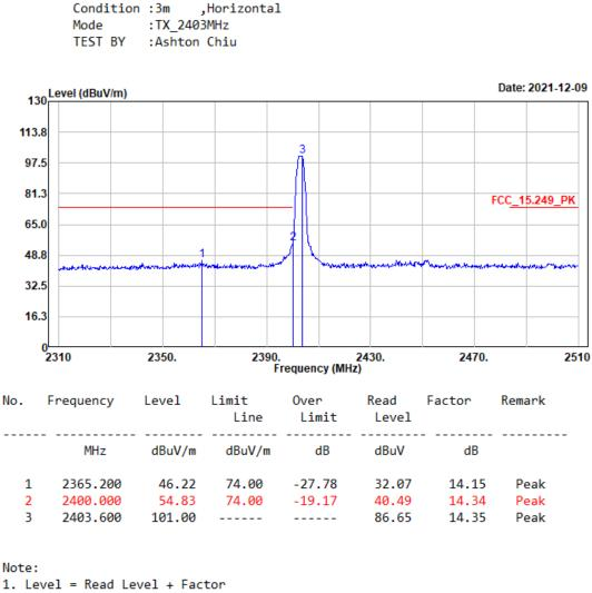
2. Factor = Antenna Factor + Cable Loss - Preamp Factor
