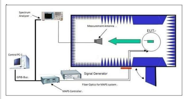
Figure 1. 2D antenna pattern test system.
