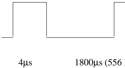
The frequency of the pulse is 556Hz, giving a period of ~1.8 milliseconds. The on time is 4 $\mu$ s, so then the averaging factor is
