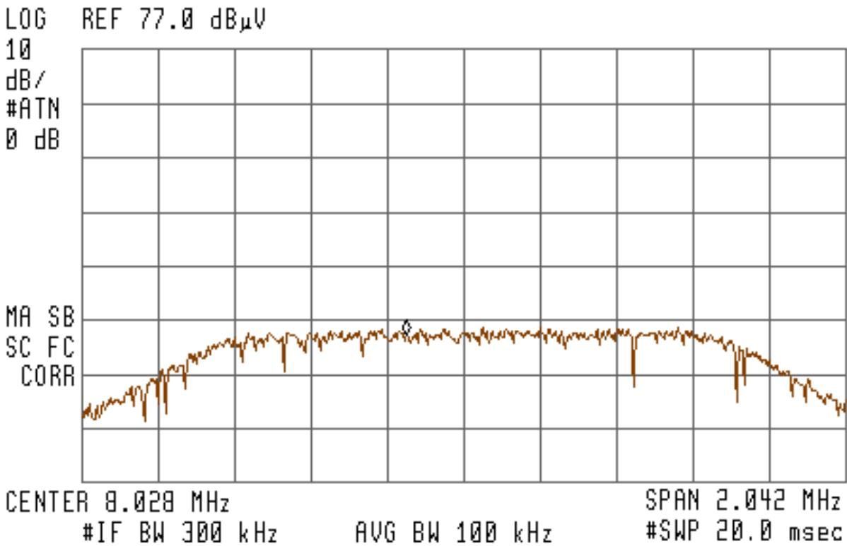
The peak measurement is 25.4 dB $\mu$ V, with cable loss of 0.6 dB, and an antenna factor of 9.4 dB. Additionally, a duty cycle factor of 20 dB can be applied. The duty cycle calculation can be found in Section X.
