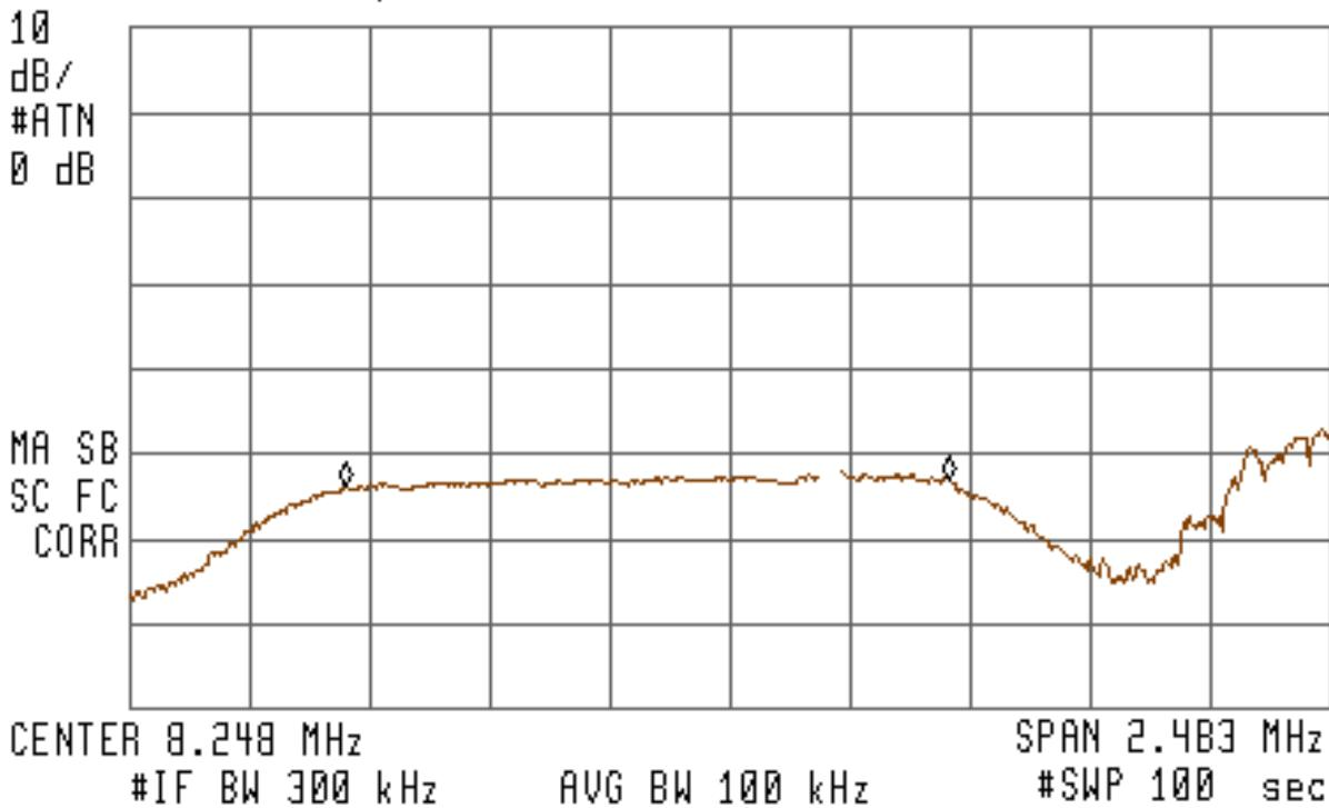
The bandwidth between the lowest and highest transmission frequency is 1.247 MHz.
