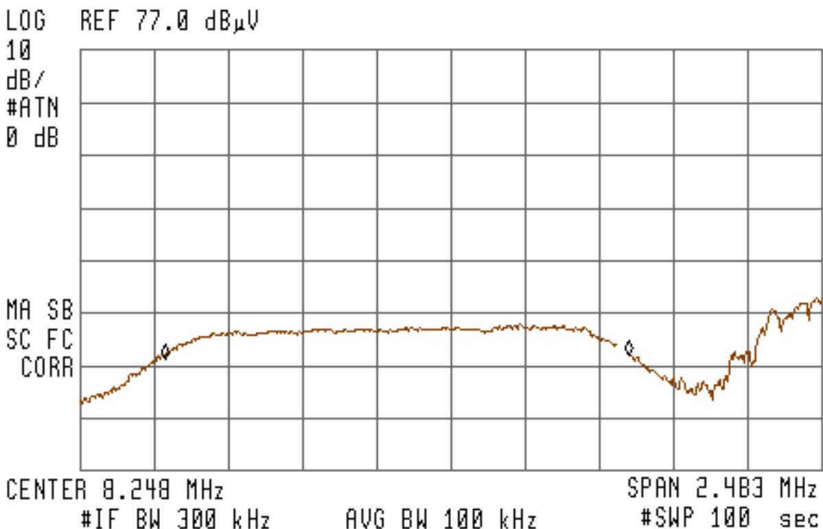
The 6 dB bandwidth of the fundamental emission is 1.552 MHz. This is 19.7% of the fundamental frequency, which is 7.873 MHz.
