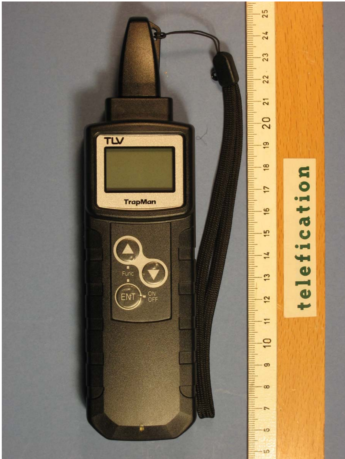
Photograph 1: - Steam Trap Management System, model TM6, front view
