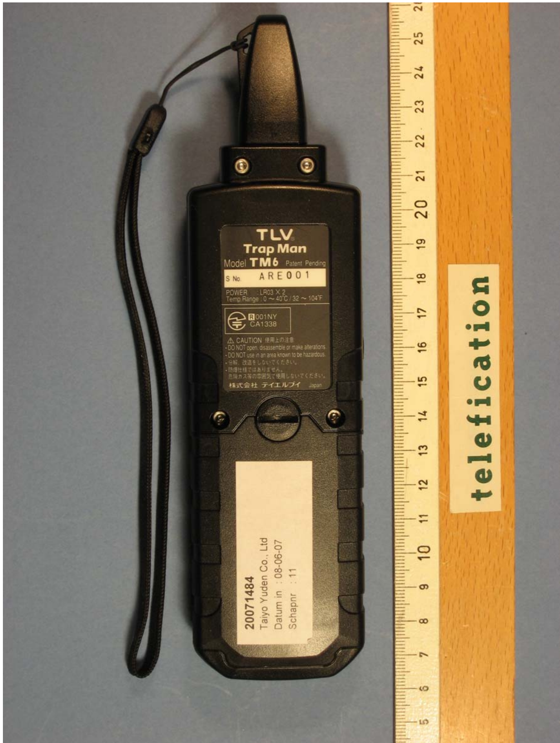
Photograph 2: - Steam Trap Management System, model TM6, rear view
