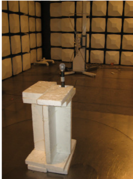
Picture 1: Spurious Radiation Measurement, 30MHz-1GHz
