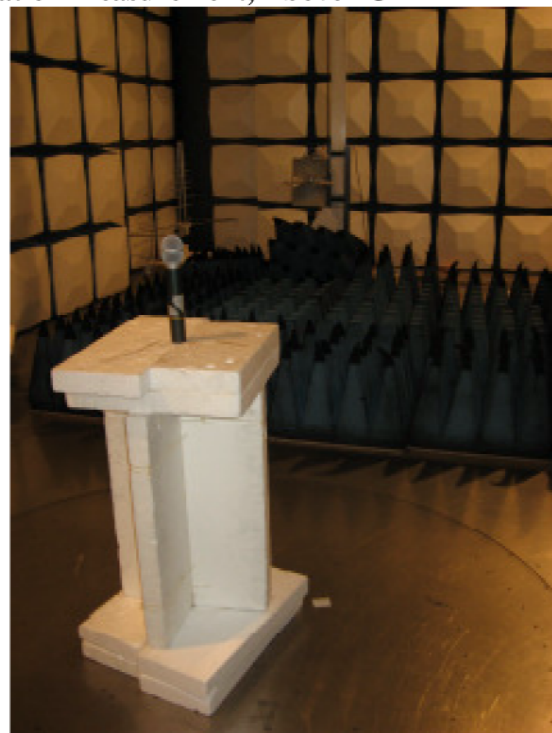
Picture 2: Spurious Radiation Measurement, Above 1GHz
