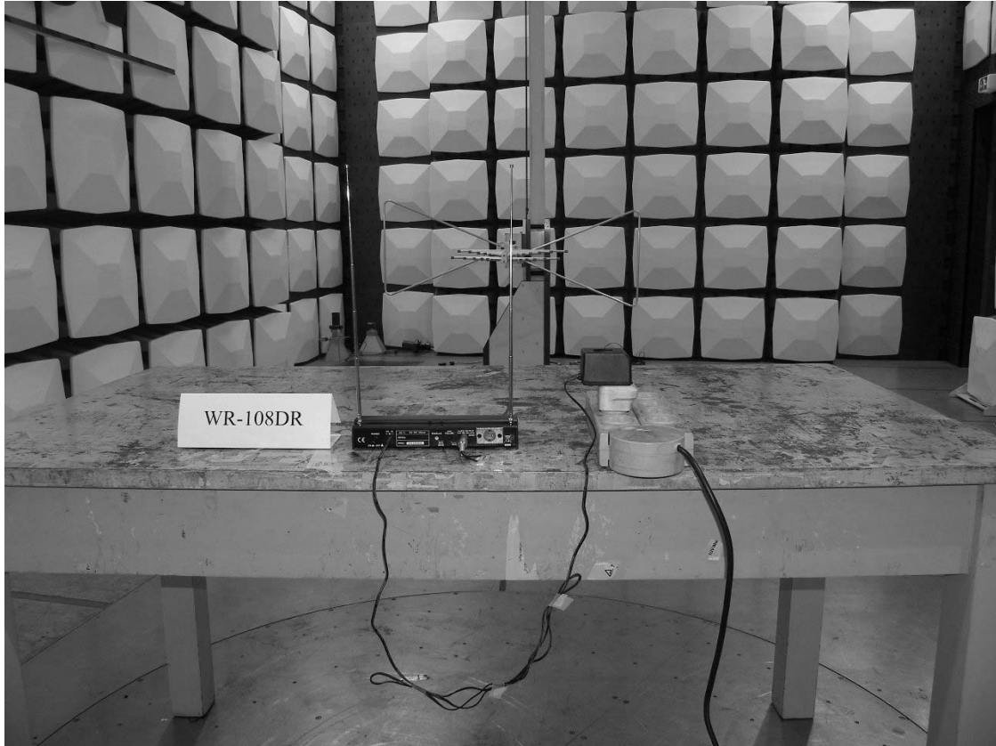
Photograph 2: Set-up for Radiation Measurement Below 1GHz
