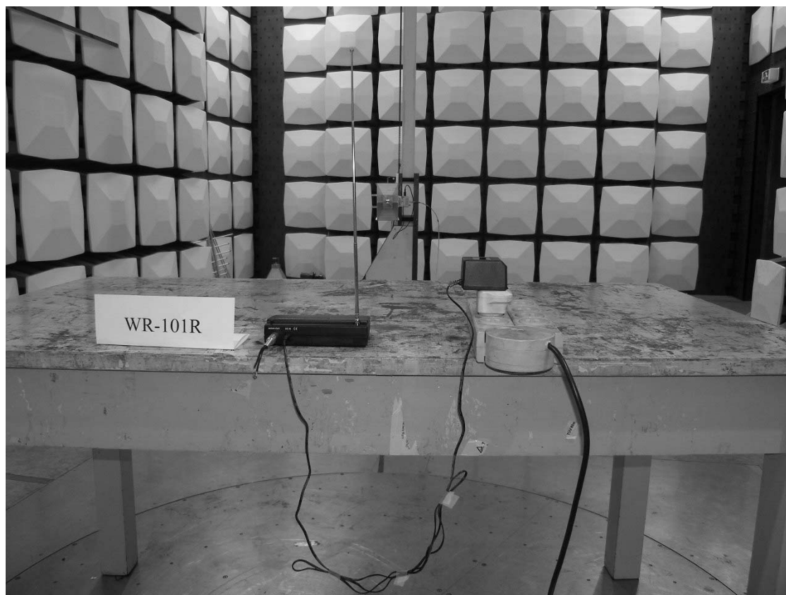
Photograph 3: Set-up for Radiation Measurement Above 1GHz
