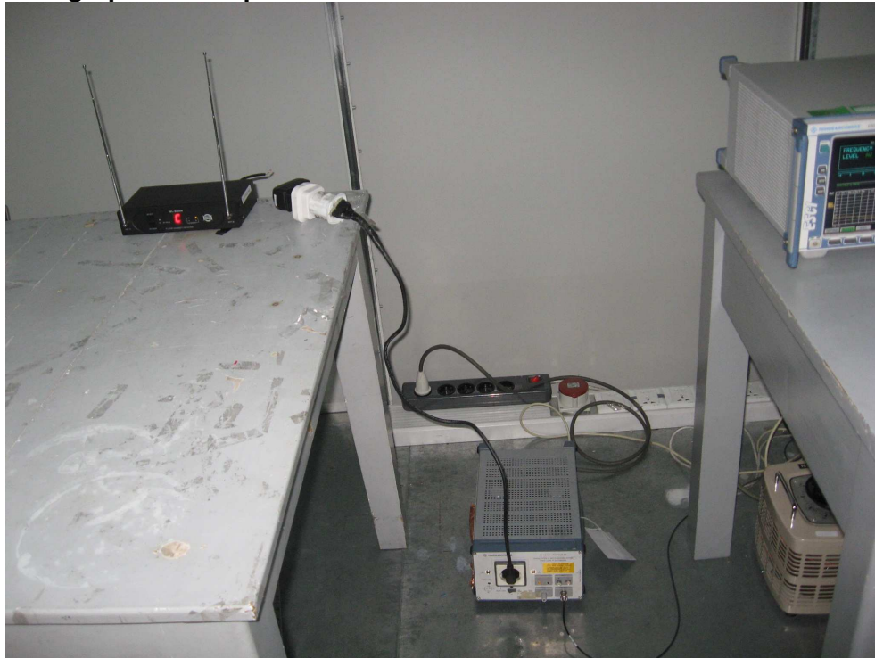
Photograph 2: Set-up for Radiated Emissions, below 1GHz
