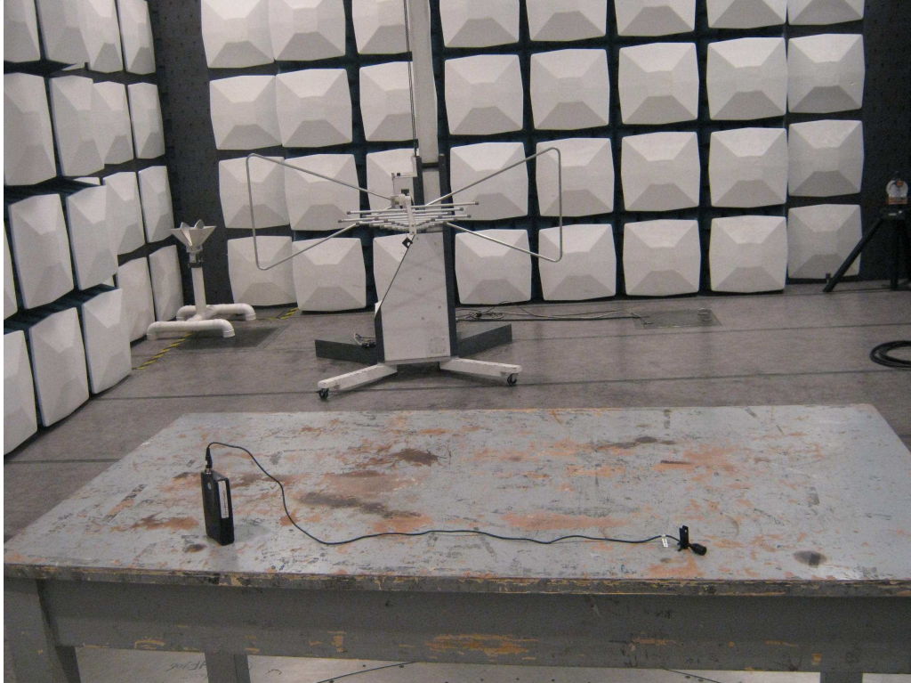
Photograph 2: Set-up for Spurious Emissions (1GHz-5GHz)
