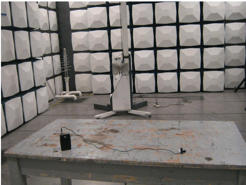
Photograph 2: Set-up for Spurious Emissions (1GHz-5GHz)
