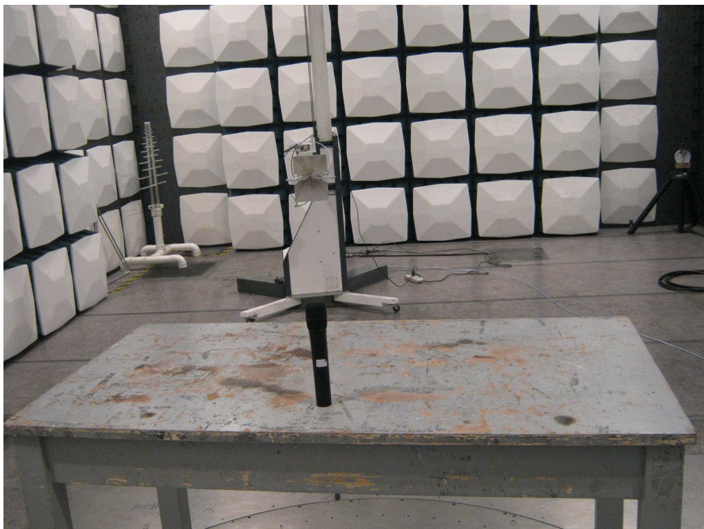
Photograph 2: Set-up for Spurious Emissions (1GHz-5GHz)
