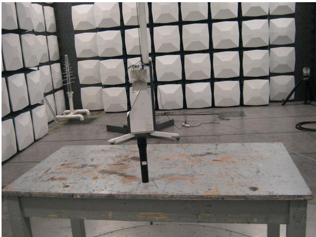
Photograph 2: Set-up for Spurious Emissions (1GHz-5GHz)
