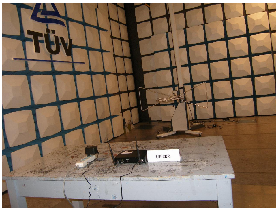
Photograph 2: Set-up for Radiation Measurement Below 1GHz
