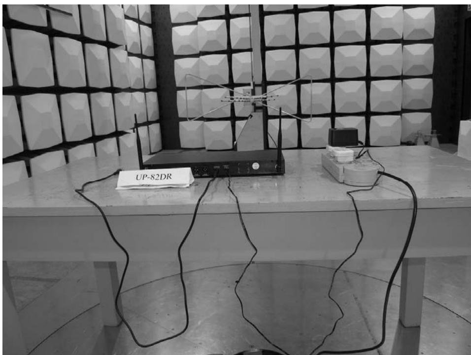
Photograph 2: Set-up for Radiation Measurement Below 1GHz
