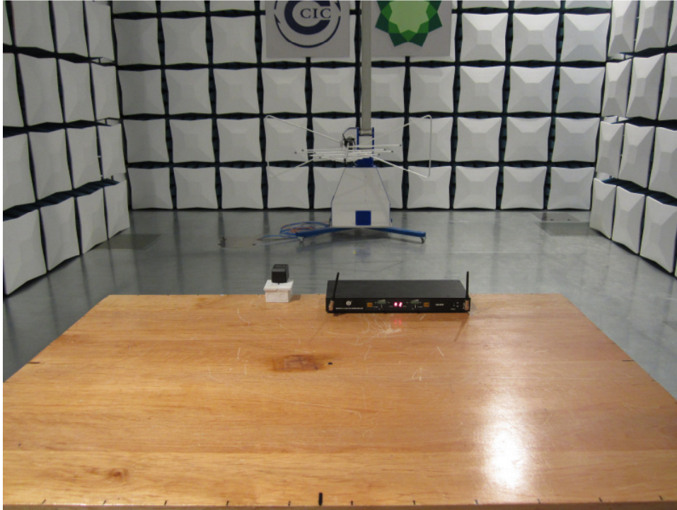
Photograph 5: Set-up for Radiated Emissions below 1GHz, model UB-82R
