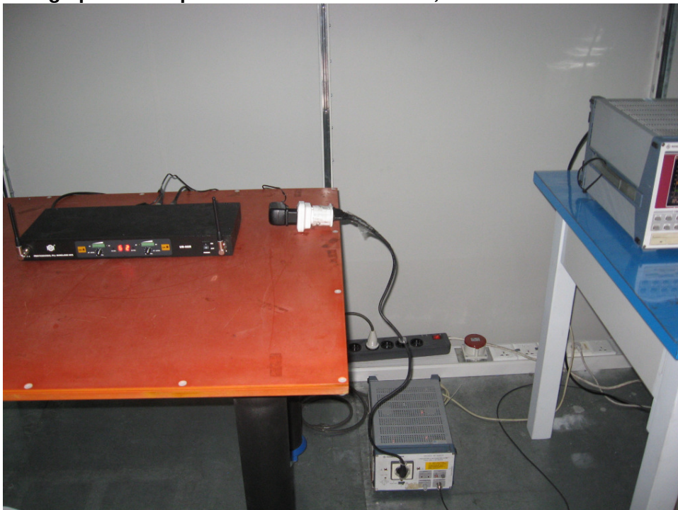
Photograph 4: Set-up for Conducted Emissions, model UB-82R
