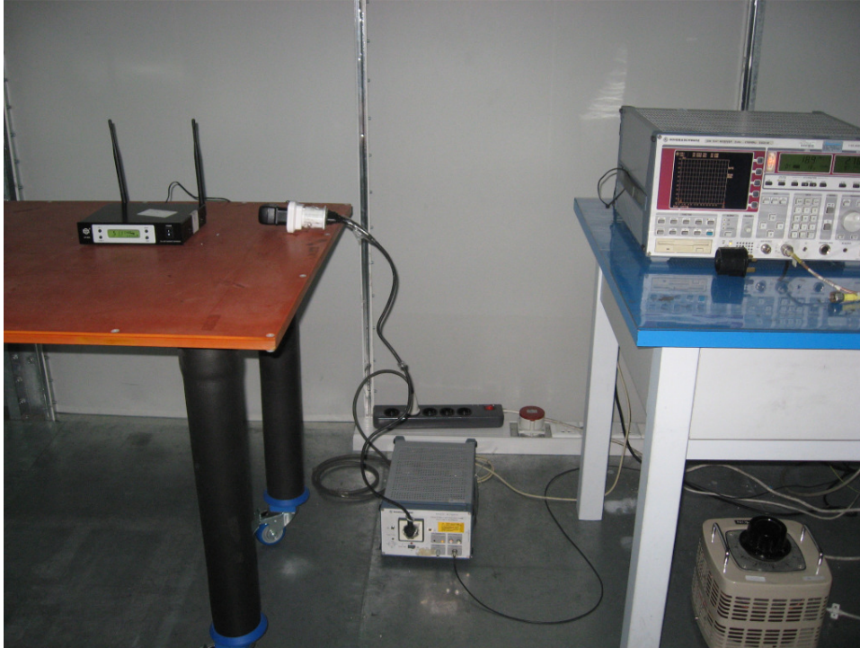
Photograph 2: Set-up for Radiated Emissions below 1GHz, model UP-8DR
