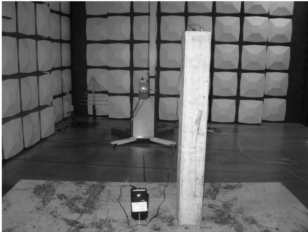
Photograph 2: Set-up for Radiation Measurement Above 1GHz
