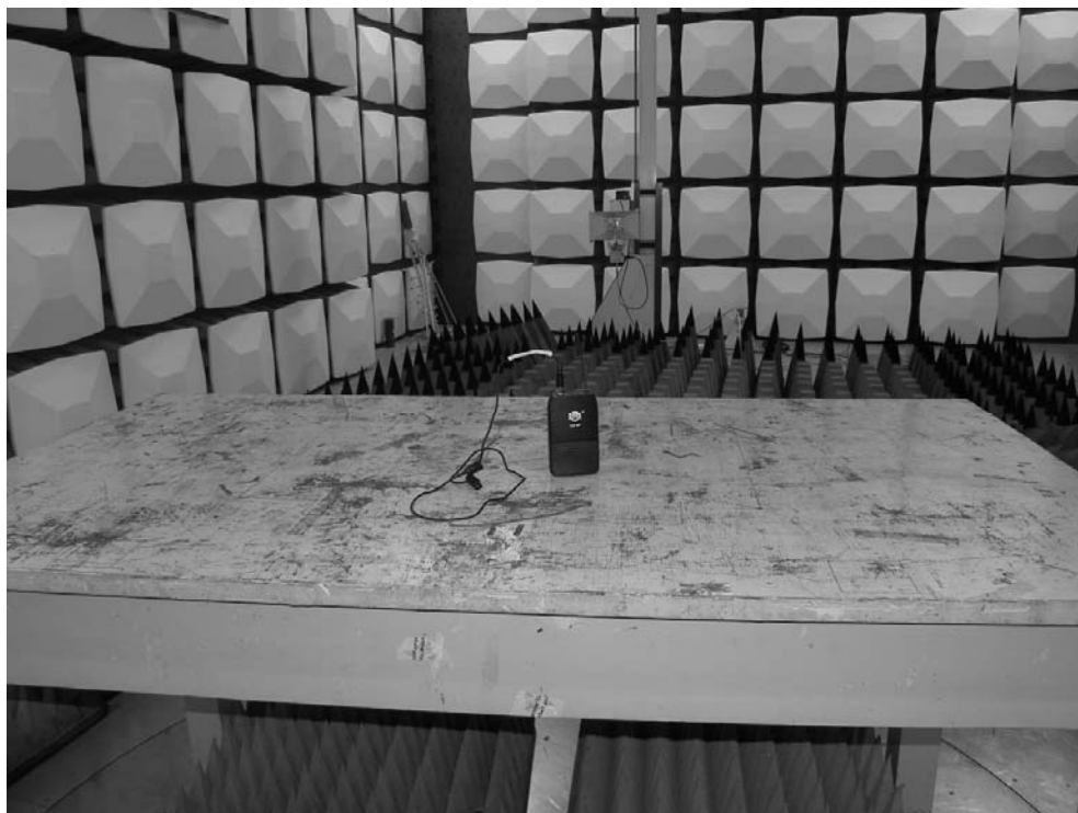
Photograph 2: Set-up for Radiation Measurement above 1GHz
