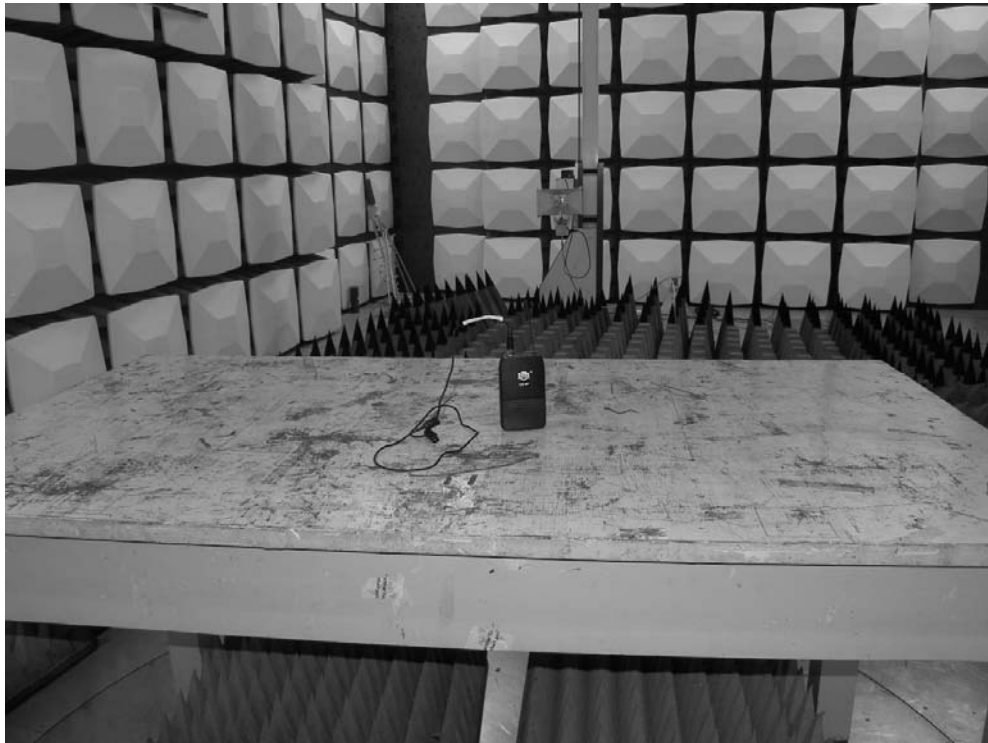
Photograph 2: Set-up for Radiation Measurement above 1GHz
