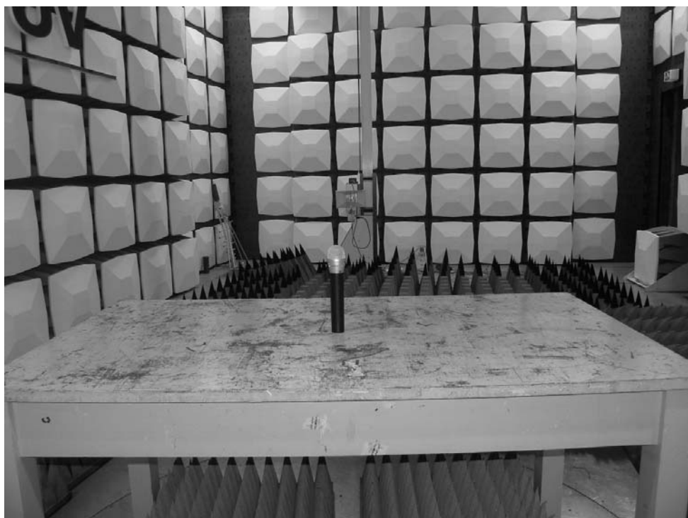
Photograph 2: Set-up for Radiation Measurement above 1GHz
