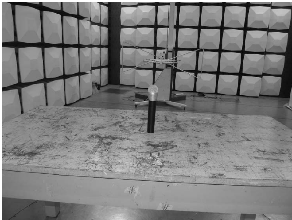
Photograph 1: Set-up for Radiation Measurement Below 1GHz
