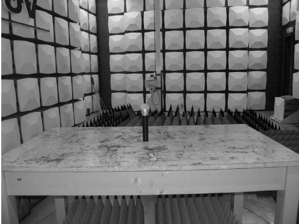
Photograph 2: Set-up for Radiation Measurement above 1GHz
