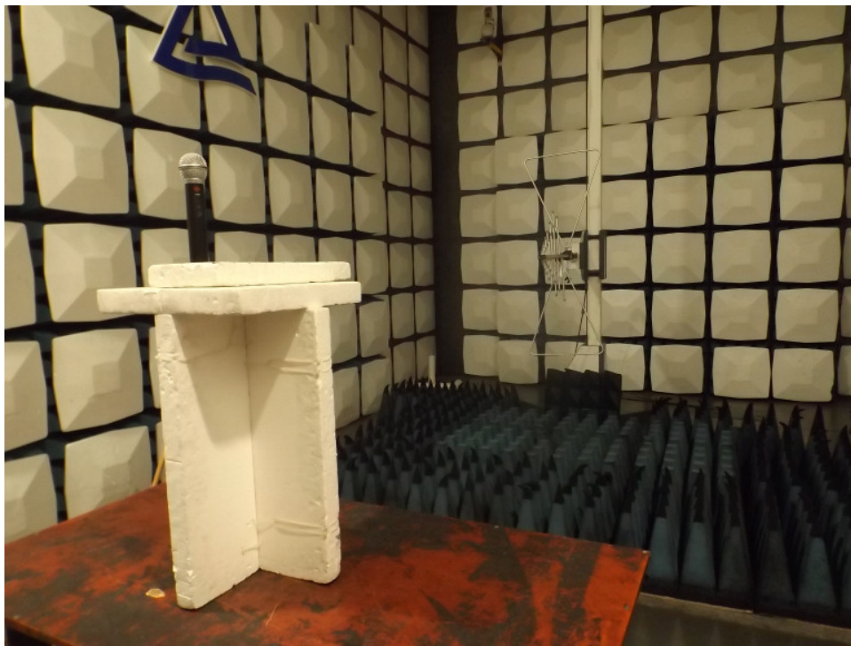
Picture 2: Spurious Radiation Measurement, Above 1GHz (U-299H)
