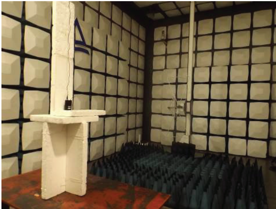
Picture 2: Spurious Radiation Measurement, Above 1GHz (U-899P)
