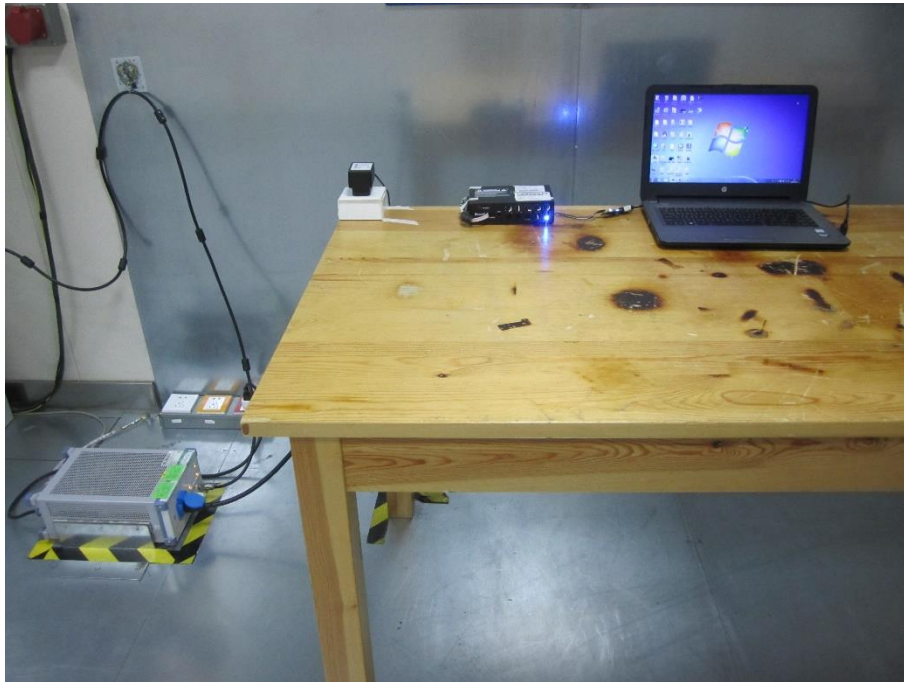
Photograph 3: Set-up for Conducted Emission on AC Mains
