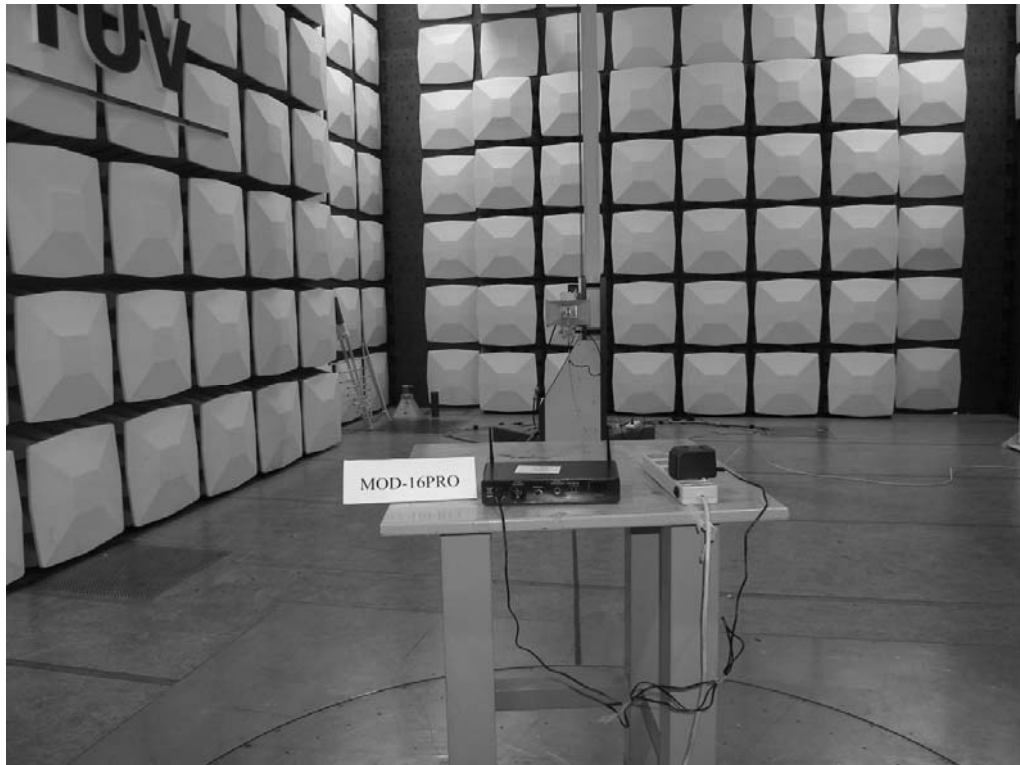
Photograph 3: Set-up for Radiation Measurement Above 1GHz
