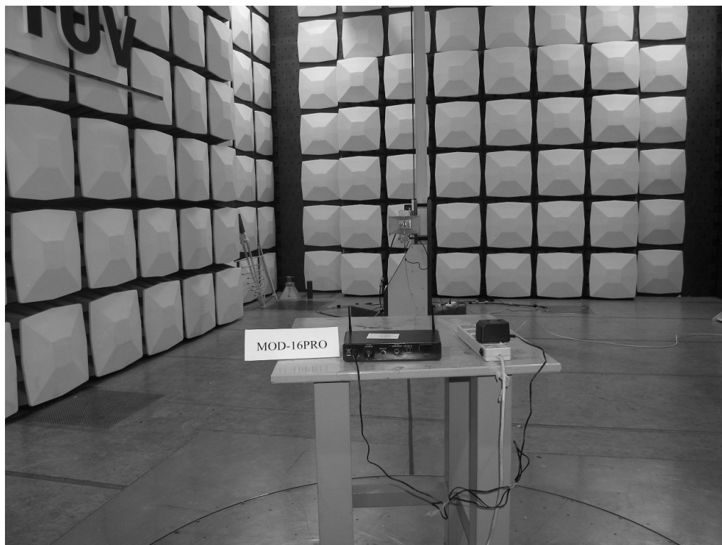
Photograph 3: Set-up for Radiation Measurement Above 1GHz
