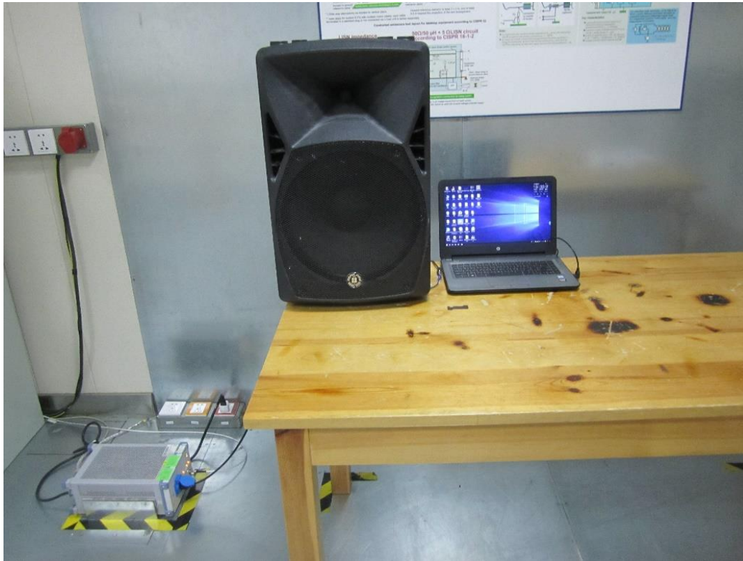
Photograph 3: Set-up for Conducted Emission on AC Mains
