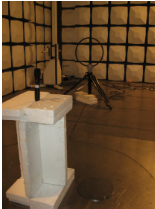
Photograph 1: Set-up for Radiation Measurement below 1GHz
