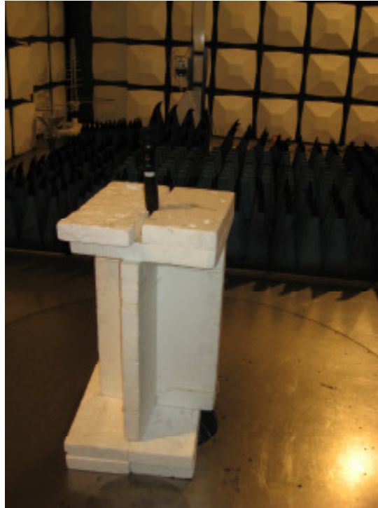
Photograph 2: Set-up for Radiation Measurement above 1GHz
