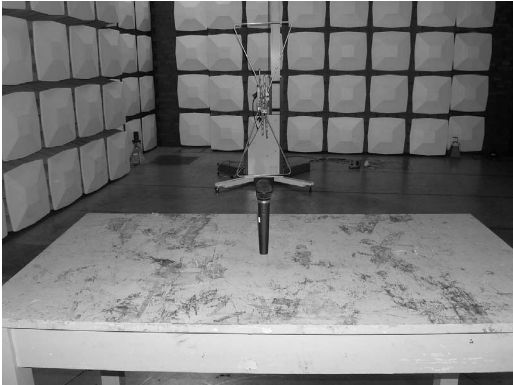
Photograph 1: Set-up for Radiation Measurement Below 1GHz
