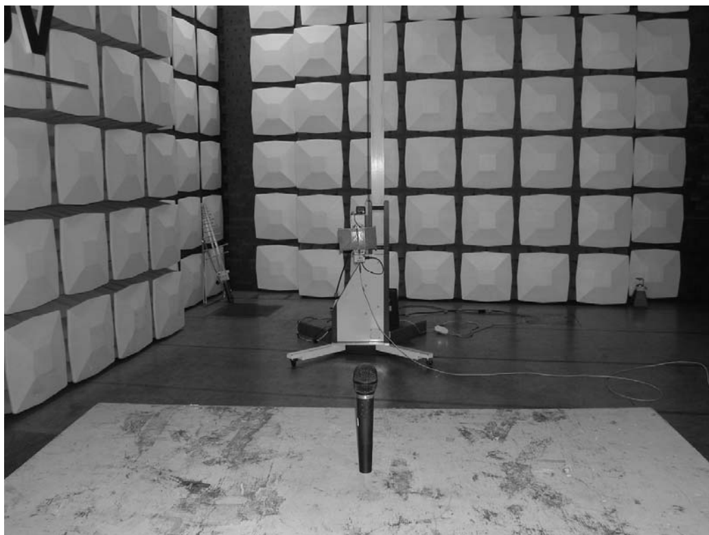
Photograph 2: Set-up for Radiation Measurement above 1GHz
