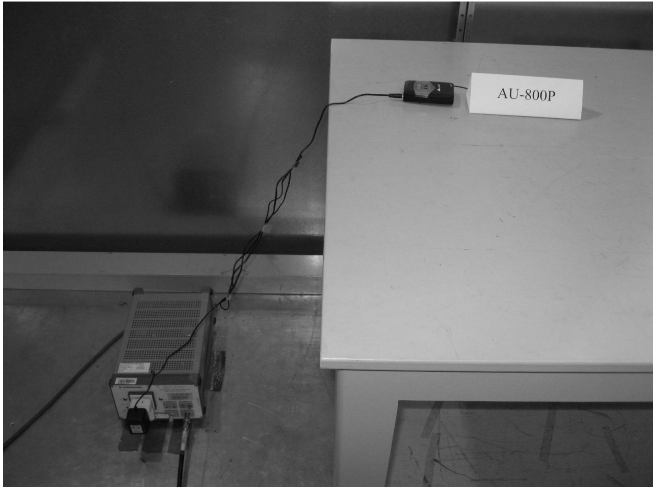
Photograph 3: Set-up for Conducted Emission of AC mains
