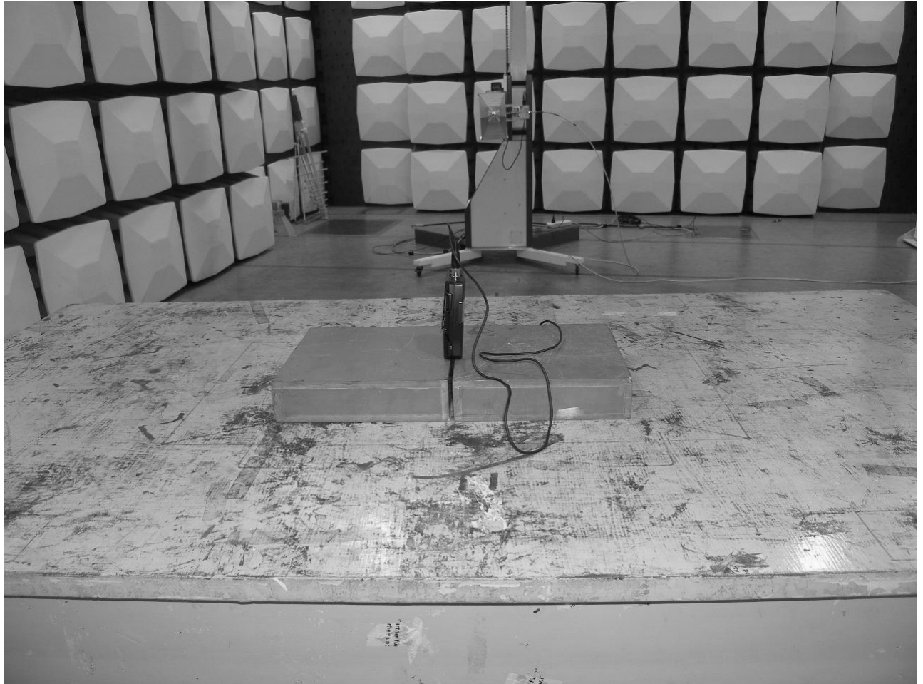
Photograph 2: Set-up for Radiation Measurement above 1GHz
