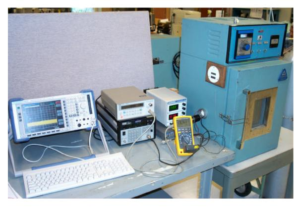
Frequency and RF power over temperature test setup:
