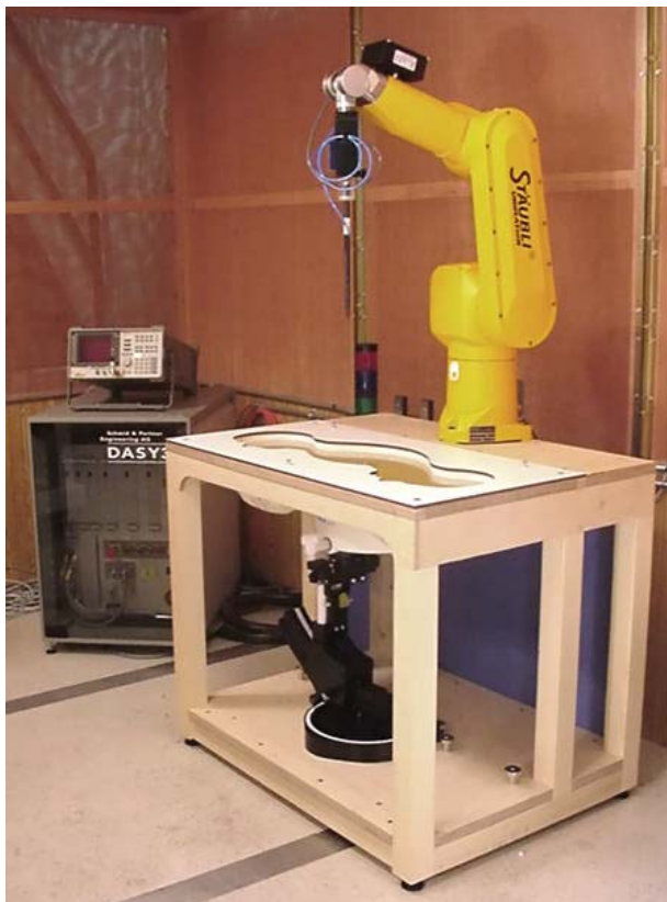
DASY3 SAR Measurement System with SAM phantom
