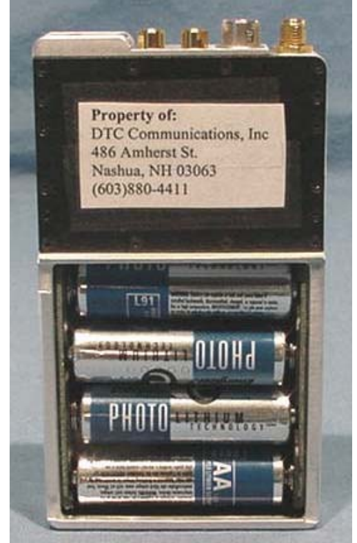
Back of Transmitter with Lithium Batteries
