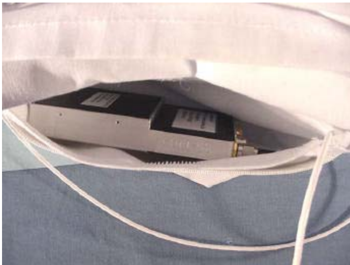
Transmitter in Vest Pouch (Velcro Open)
