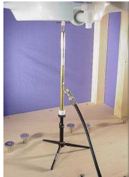
2450MHz Dipole Validation Setup
