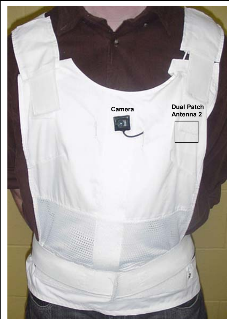
Front Side of VidiVest (P/N: 1088185) - Dual Patch Antenna 2 Location
