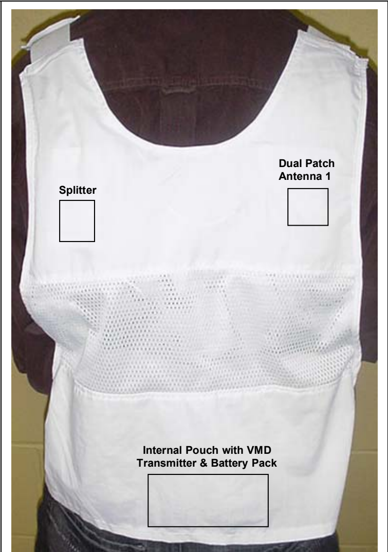
Back Side of VidiVest (P/N: 1088185) - Dual Patch Antenna 1 Location
