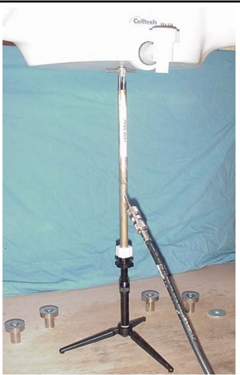
2450 MHz Validation Dipole Setup
