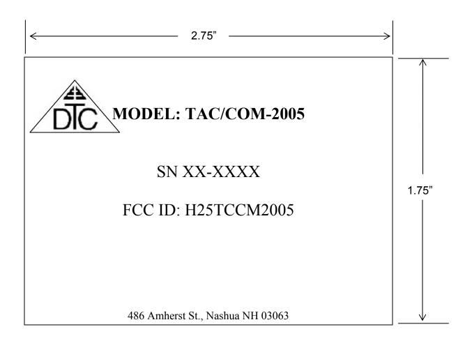
The FCC ID label is located on the device as shown in the photo.
