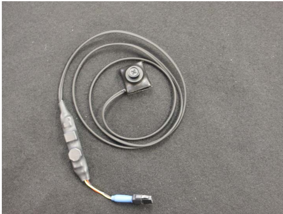
Stepdown Converter Incorporated Into Button Camera Harness
