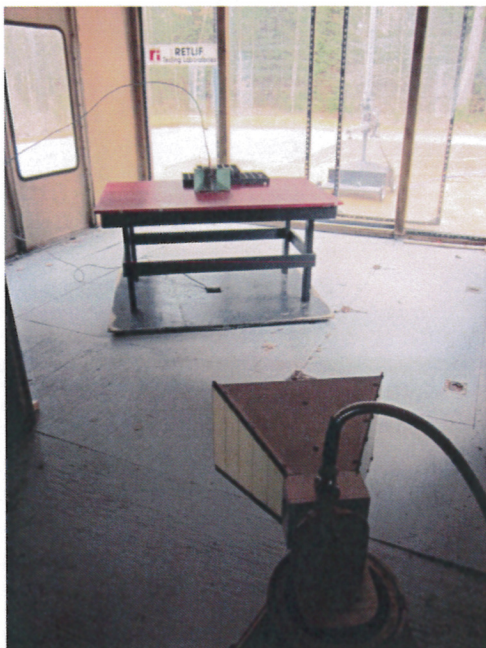
High Gain Horn Antenna, Horizontal Polarization, Substitution Antenna High Field
