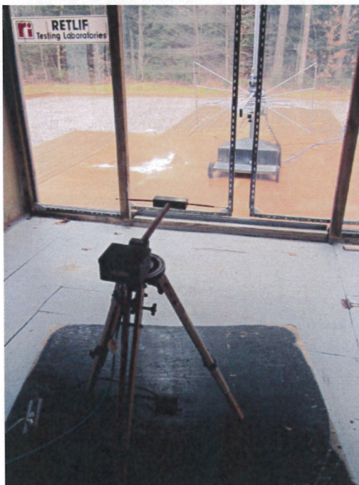
High Gain Horn Antenna, Vertical Polarization Substitution Antenna Low Field
