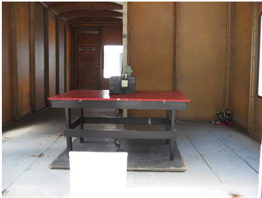
Test Setup, High Gain Horn, Vertical Antenna Polarization
