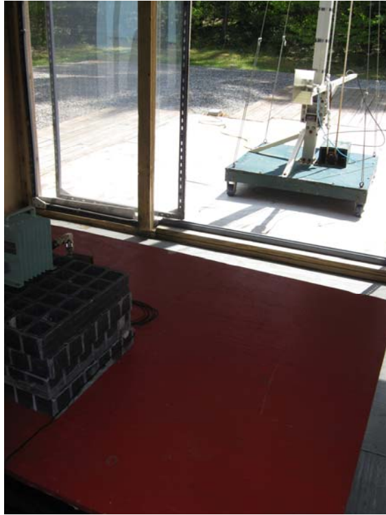
Double Ridge Guide, Horizontal Antenna Polarization
