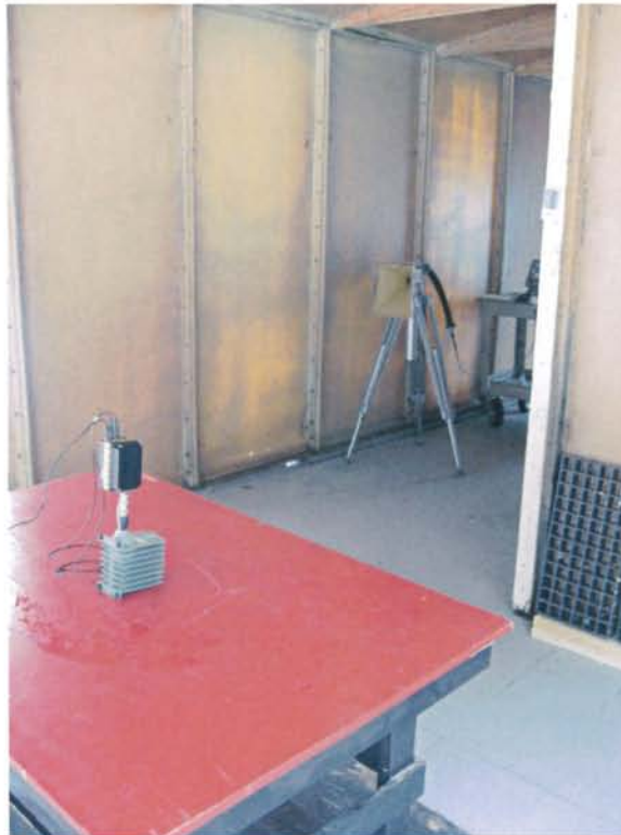
Horizontal Antenna Polarization, 5.8 to 8.2 GHz
