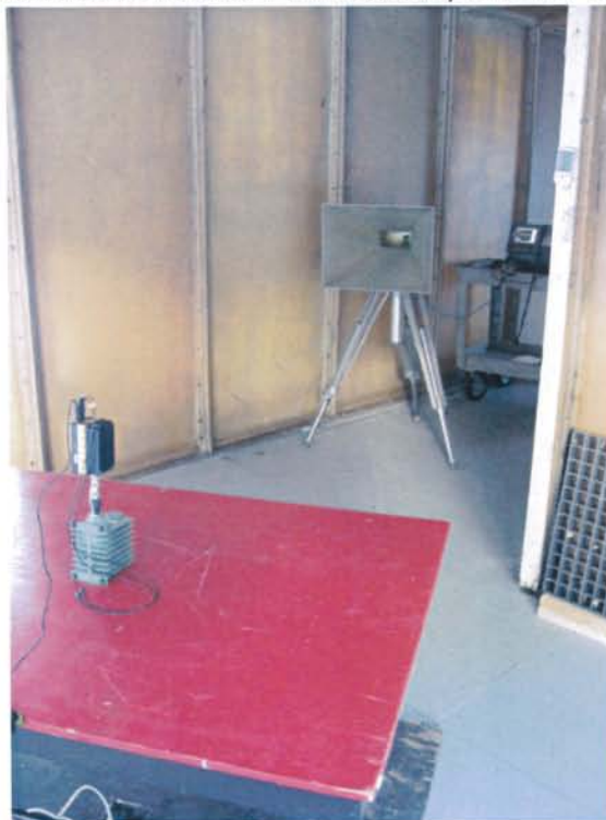
Vertical Antenna Polarization, 1 to 1.7 GHz
